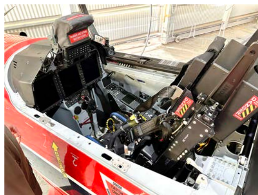
PILATUS PC 21 COCKPIT WITH THE EJECTION SEAT MECHANISM IN VIEW.
