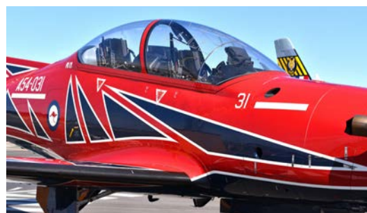
PILATUS PC 21 COCKPIT THE AIRCRAFT HAS TWO CREW THE PILOT IN TRAINING AND THE INSTRUCTOR SITS BEHIND.
