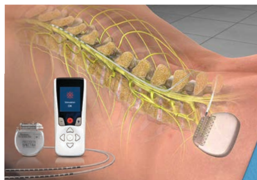
THE BOSTON SCIENTIFIC SPINAL CORD STIMULATOR (SCS) IS A DEVICE DESIGNED TO HELP MANAGE CHRONIC PAIN BY SENDING ELECTRICAL IMPULSES TO THE SPINAL CORD, WHICH BLOCKS PAIN SIGNALS FROM REACHING THE BRAIN.
